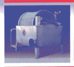
The KEMCO Rotary Filter effectively removes wastewater particulate and offers easy operation with minimum maintenance. A unique rotating screen drum produces trouble-free operation as the raw wastewater flows through the filter.
